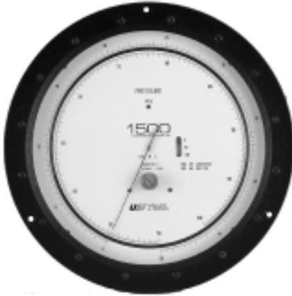
Series 1500 Gauges have capsule-type pressure elements up to and including the 150-psig range. Ranges of 200 psig and above have Bourdon tubes. The pressure to be measured is applied to the capsule or Bourdon tube through a single connection in the case. The case has a tempered-glass dial cover, solid-front dial, and a blow-out plug on the back. Readings are referred to atmospheric pressure in the case.
