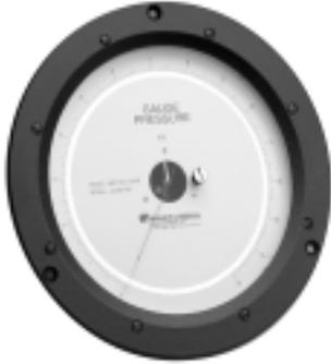
For routine test and production uses, this capsule-type gauge offers an acceptable balance among size, readability, accuracy, and price. Available in 18 standard ranges (including vacuum and compound ranges), the Series 300 is convenient to use. High differential pressure is applied to the capsule; low pressure to the case. Maximum static (case) pressure is 15 psig. A built-in overpressure relief valve protects the case.
