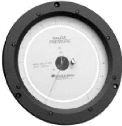
For routine test and production uses, this capsule-type gauge offers an acceptable balance among size, readability, accuracy, and price. Available in 18 standard ranges (including vacuum and compound ranges), the Series 300 is convenient to use. Pressure is applied to the capsule through a single connection in the case. Readings are referenced to atmospheric pressure in the case.
